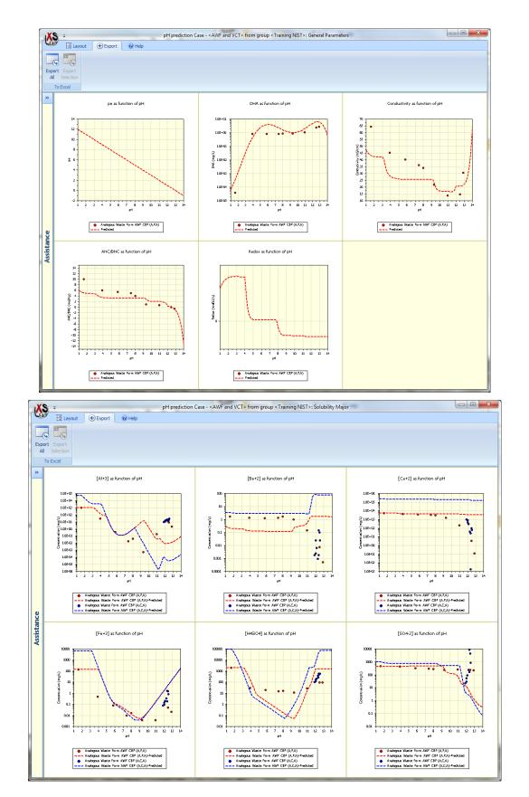
The red dots are the pH dependent leaching test data (Method 1313). The blue dots are the percolation test data (Method 1314). If the data overlap, the conclusion is that the substance is solubility controlled and pH and redox are more important controlling factors of release than L/S (liquid to solid ratio).
