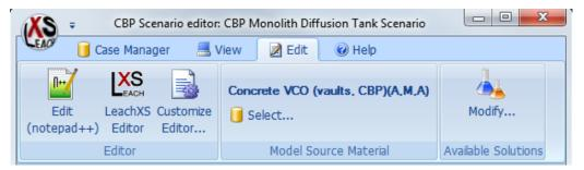
Tab group Model Source Material will only be present if you have opened a scenario for simulating a lab test. By pressing the Select... button you can select an existing lab test. The geometry and other physical parameters of the model will be set to the geometry and physical parameters of your selected test.
